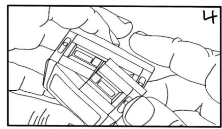
Tuck in place. Repeat on front bumper, passenger side first then driver side.
